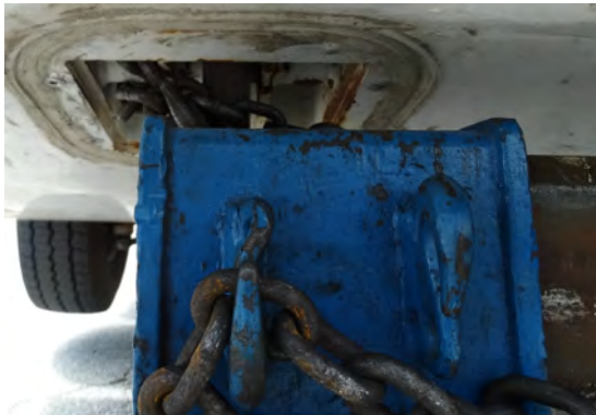
Figure 1-17. Install Tow Fork Safety Chains
