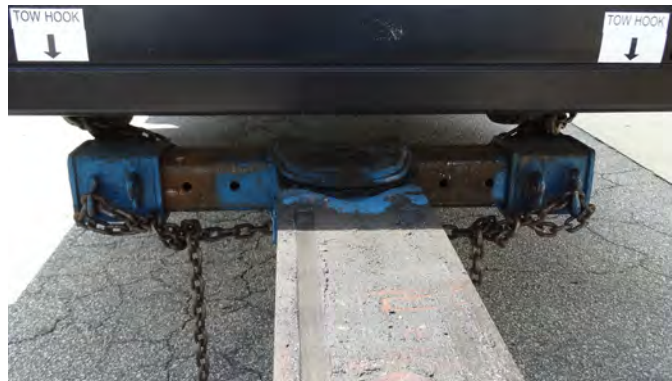
Figure 1-17. Install Tow Fork Safety Chains
