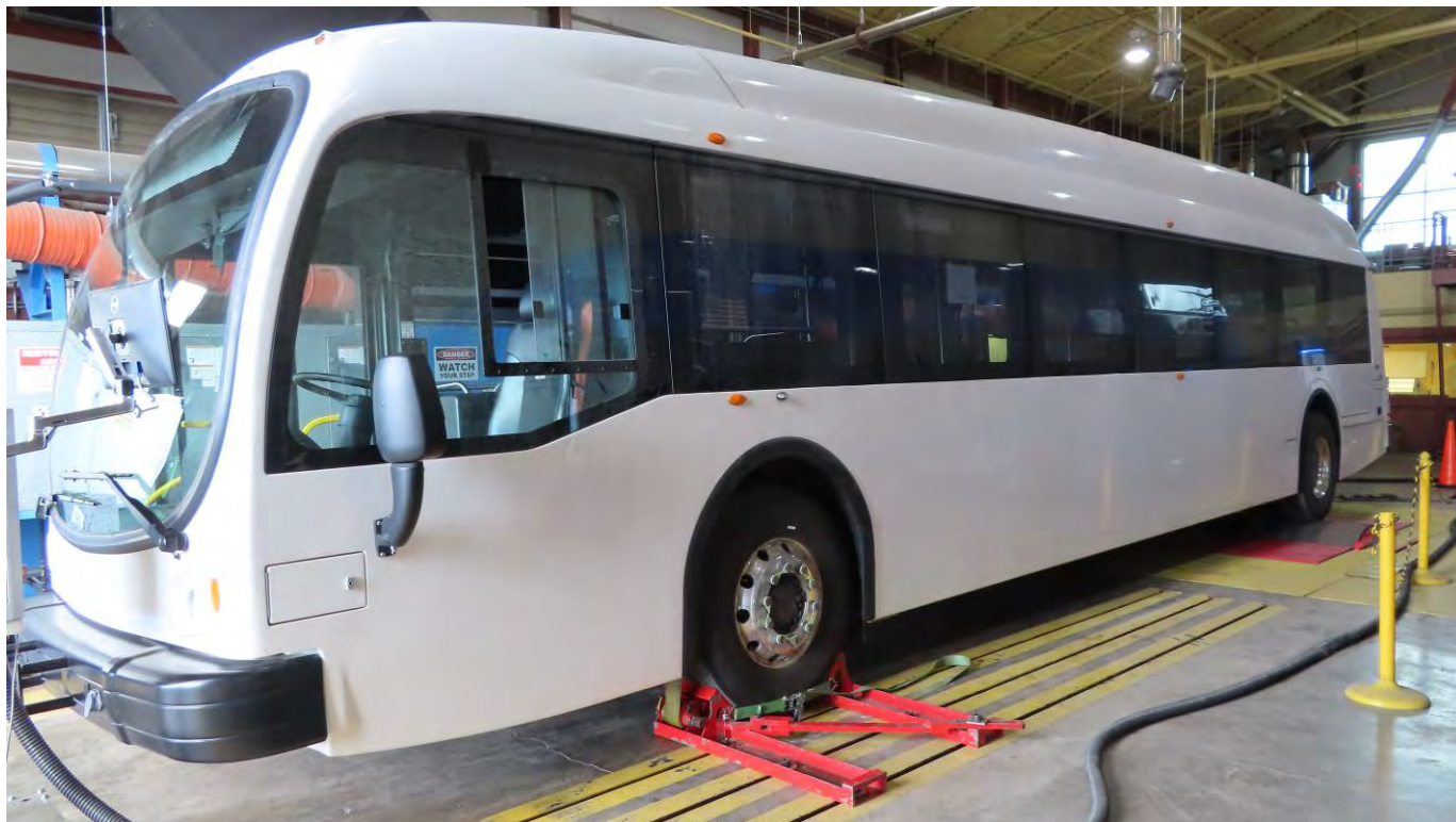
BUS TESTED ON CHASSIS DYNAMOMETER FOR PERFORMANCE AND ENERGY ECONOMY
