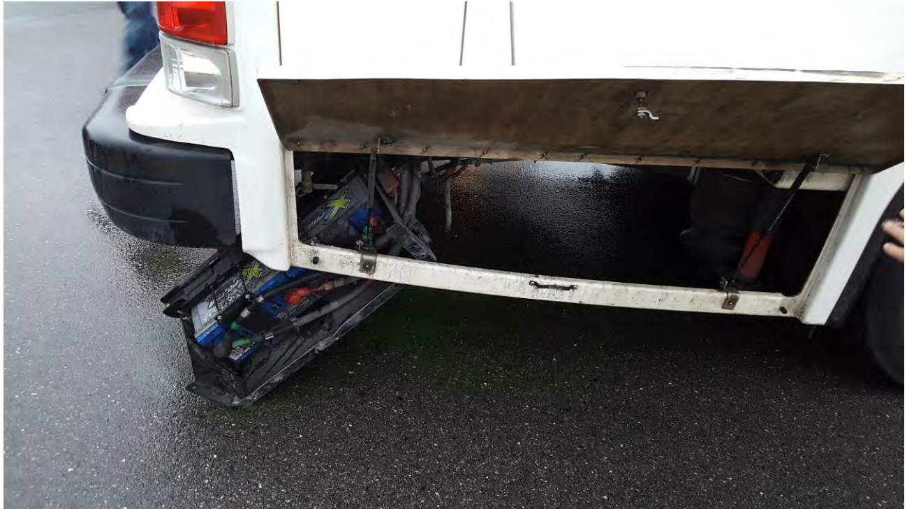
24 VOLT BATTERY BOX FELL OUT (9,334 TEST MILES)
