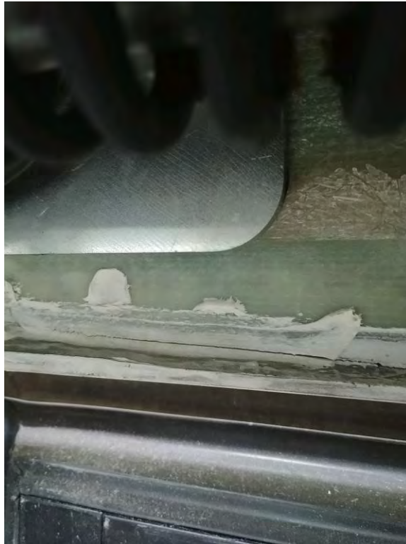
CRACKS AROUND REAR DOOR (12,999 TEST MILES)
