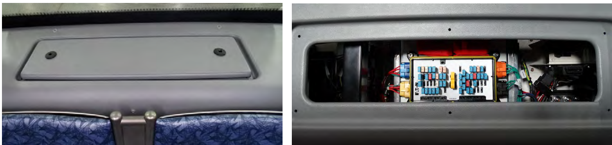
Figure 1-4. Opening the Rear Deck Access Covers
