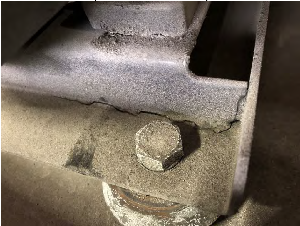
AIR COMPRESSOR BRACKET IS CRACKED (12,598 TEST MILES)
