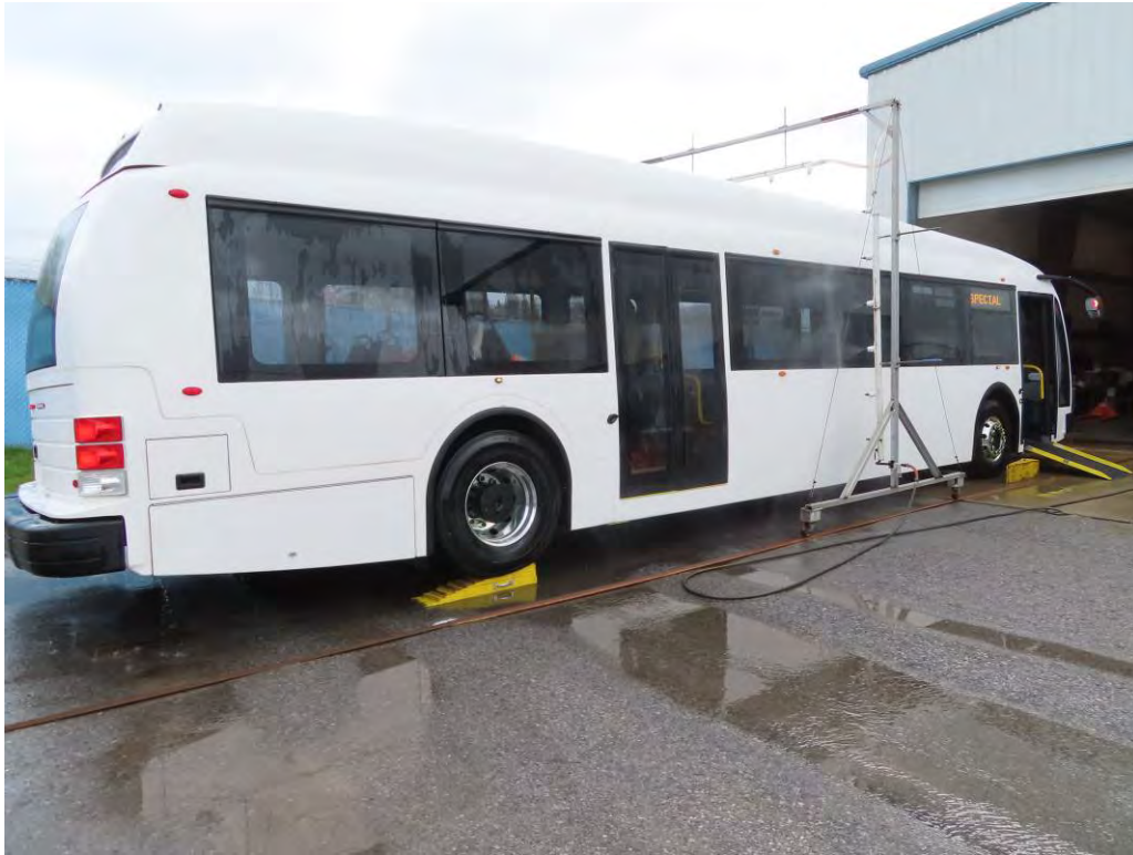
RIGHT REAR WHEEL SIX INCHES HIGHER
