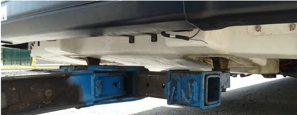
Figure 1-16. Lift the Bus
