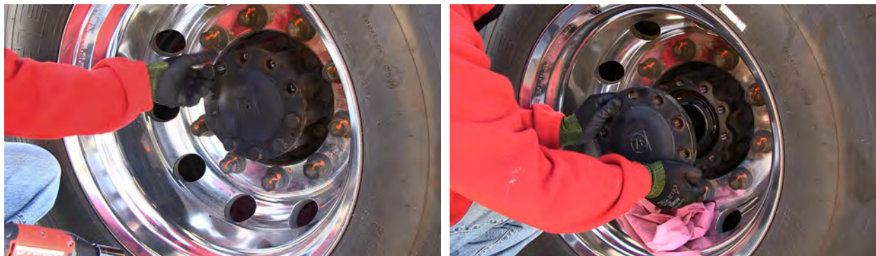
Figure 1-20. Removing the Half Shaft
