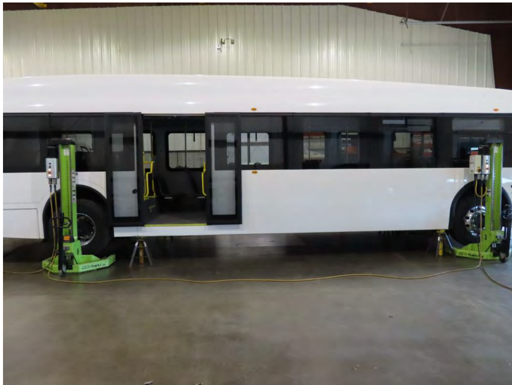
FRONT AND REAR JACK STANDS IN PLACE
