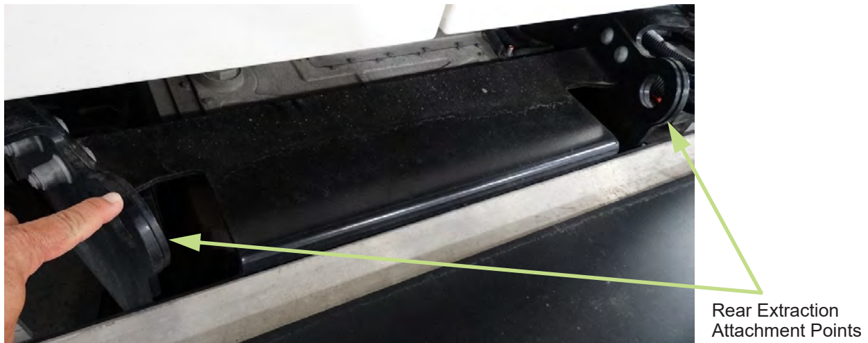
Figure 1-11. Rear Extraction Points on ProDrive Frame
