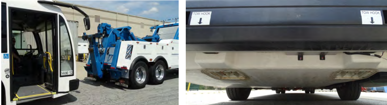
Figure 1-13. Tow Truck Positioned for Front Extraction
