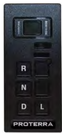
Figure 2: Gear selector layout with D and L buttons
