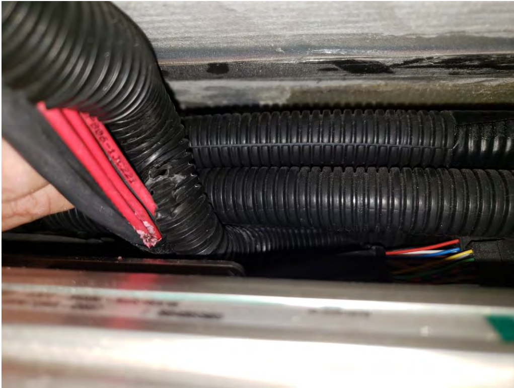
REAR DOOR LOW VOLTAGE HARNESS IS CHAFFING (6,511 TEST MILES)
