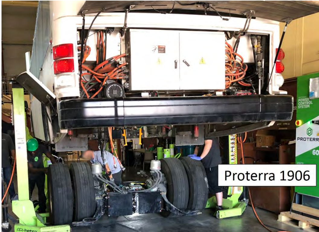
DUOPOWER AXLE REMOVAL AND REPLACEMENT (4.00 LABOR HOURS)
