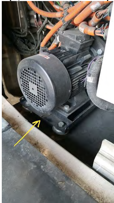
AIR COMPRESSOR BRACKET IS BROKEN (1,648 TEST MILES)
