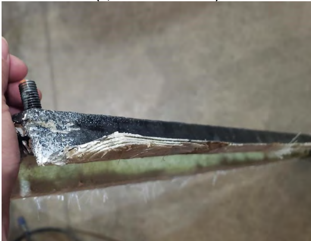
DAMAGED FRONT DOOR HAT BRACKET (6,494 TEST MILES)
