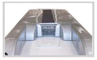
CNG Tank Valves Centrally Located for Ease of Servicing
