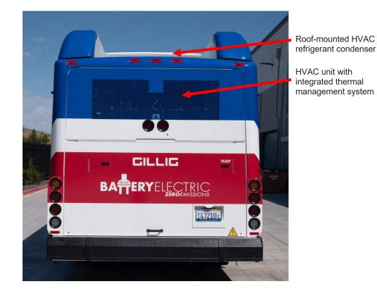
Air conditioning systems use a refrigerant that changes states between a liquid and a gas at different places in the system. The liquid refrigerant absorbs a great amount of heat when it boils and becomes a gas. When this gas is compressed and condensed back to a liquid state, the absorbed heat is given up. With the proper closed system of evaporator,
