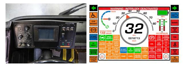
The primary screen is the default display for the driver while in motion. The relevant gauges and indicator lamps are displayed in a central location to allow the operator to quickly review the status while driving.
