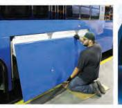
Quick-Change Skirt Panels keep the bus out of the body repair shop and back on the road for a potential collision repair savings of \$10,000/bus over 12 years.
