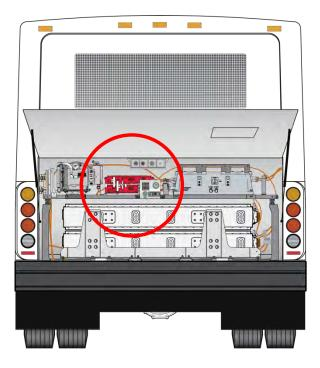
Two DC/DC converters are wired in parallel to provide the required low-voltage system capacity. The DC/DC converters are liquid-cooled by the ECP using ethylene glycol coolant.
