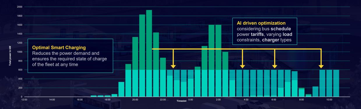
• Without SMART CHARGING the charging operations are uncontrolled and start whenever buses are plugged.
