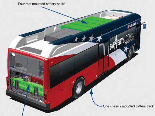
Two battery packs mounted in the powertrain compartment
