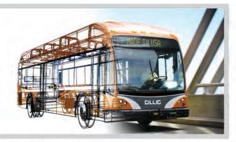
GILLIG's Low Floor body structure of lightweight, high-strength aluminum with anodized side posts resists corrosion and greatly simplifies collision repairs. Its reduced weight saves on fuel costs and its aluminum components are recyclable.
