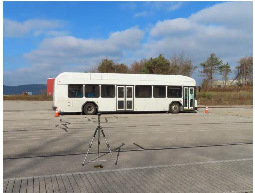
**TEST BUS UNDERGOING EXTERIOR NOISE TESTING**
