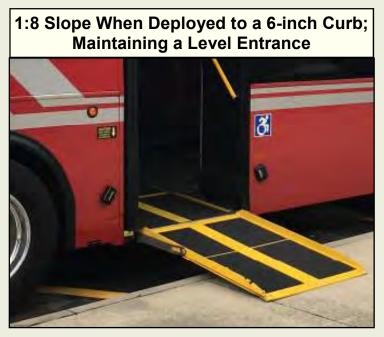
The LU18 "two-position" interior floor automatically lowers on an incline when the outer ramp reaches a pre-determined angle. Operator involvement is not required.
