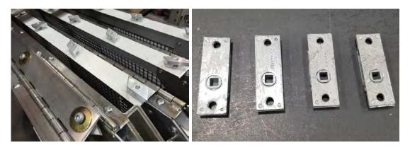
Left: Isolating tape applied over primed hinged panels. Right: Stainless steel square key locks with pre-applied protective coating.
