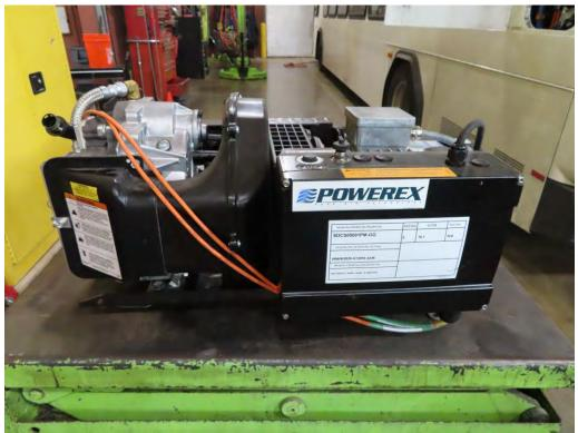
AIR COMPRESSOR REPLACEMENT (7,748 TEST MILES)
