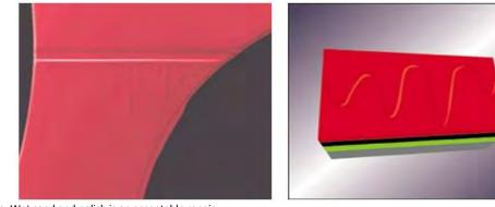
Note: Wet sand and polish is an acceptable repair.
