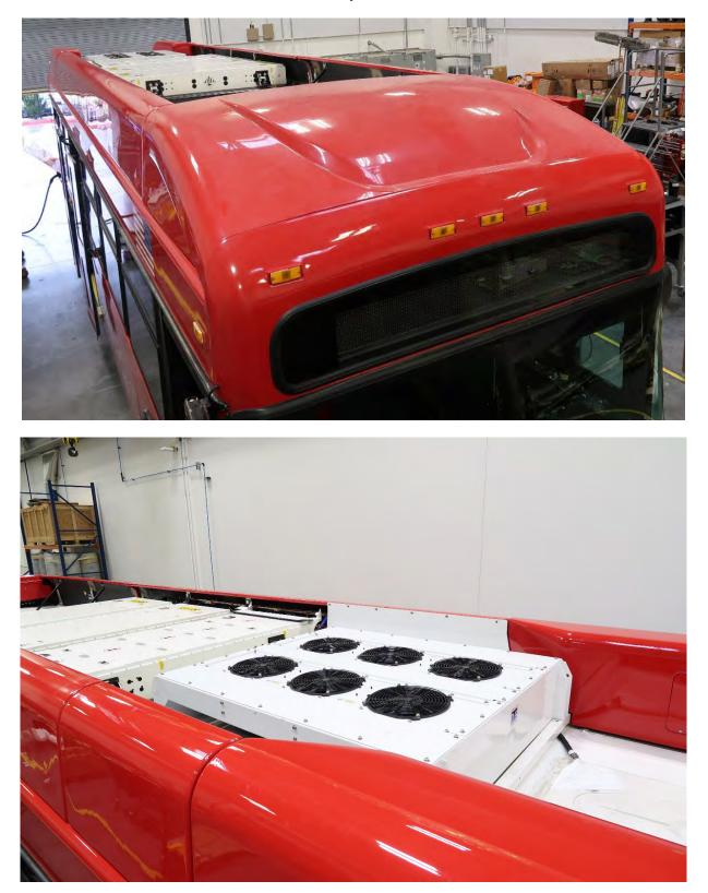
Roof Battery Installation
