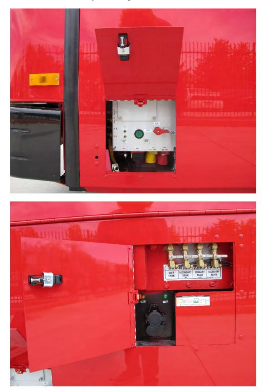
Battery Low Voltage Disconnect Switch
