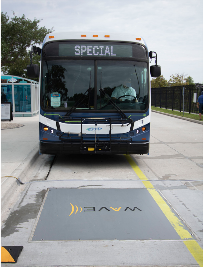
Wireless charging with inductive power transfer system at a PSTA transfer facility (Source: PSTA)
