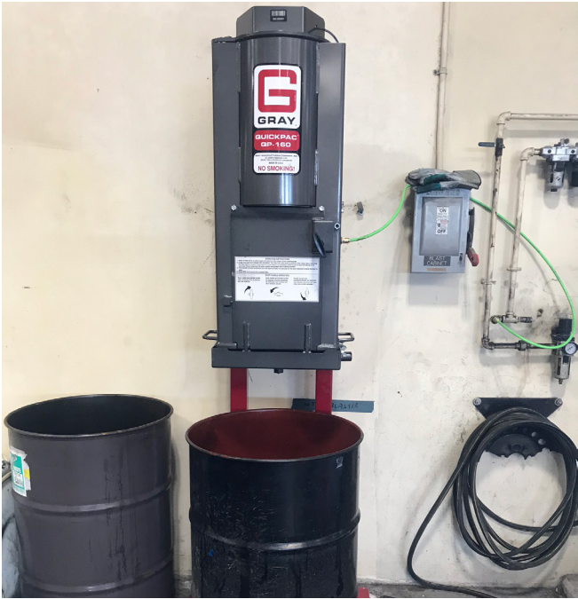
Oil filter crusher saves space in waste collection (Source: PSTA)
