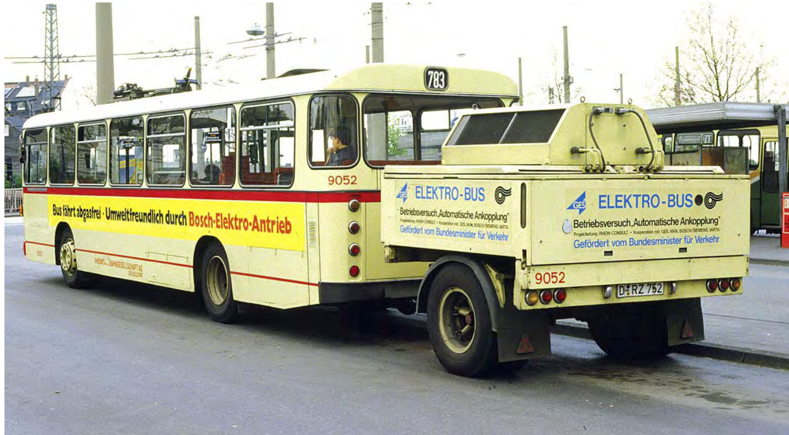
1970s German Pilot – Retrofitted Diesel Bus with Battery Trailer
