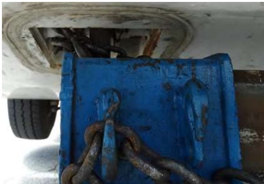
Figure 1-17. Install Tow Fork Safety Chains
