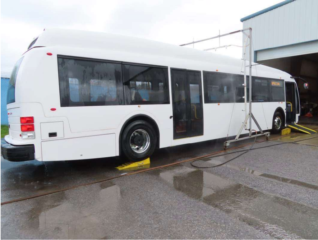
RIGHT REAR WHEEL SIX INCHES HIGHER
