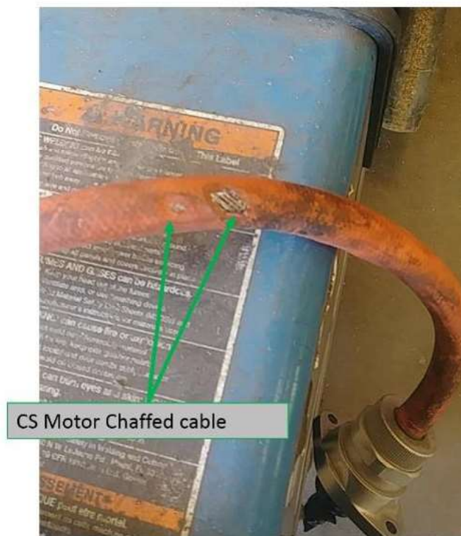
PHASE CABLE FOR CURBSIDE MOTOR IS CHAFFING (6,615 TEST MILES)
