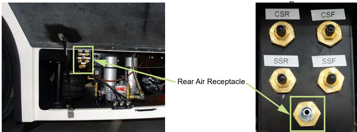
Figure 1-9. Rear Air Receptacle for Tow Truck Attachment
