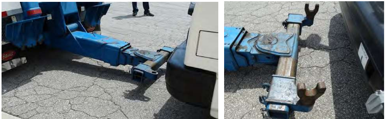
Figure 1-14. Positioning Stinger Under Front of Bus
