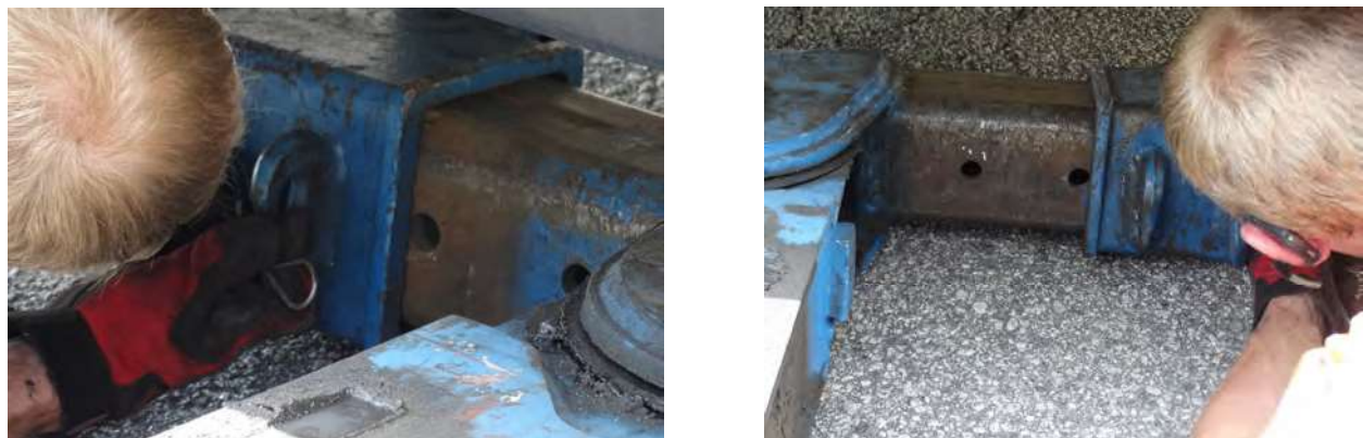
Figure 1-15. Repositioning Tow Forks to Align with Tow Pockets
