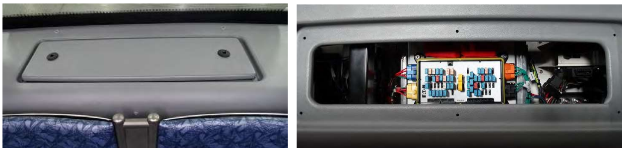
Figure 1-4. Opening the Rear Deck Access Covers
