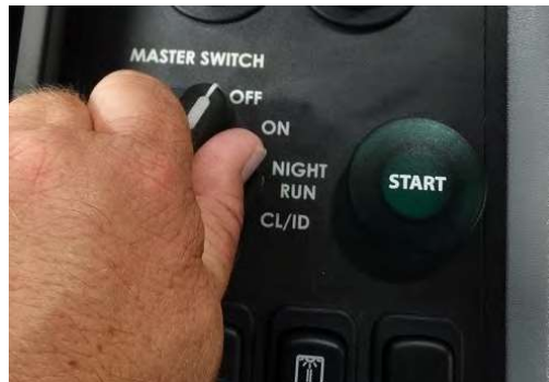
Figure 1-21. Turn ON Master Switch
