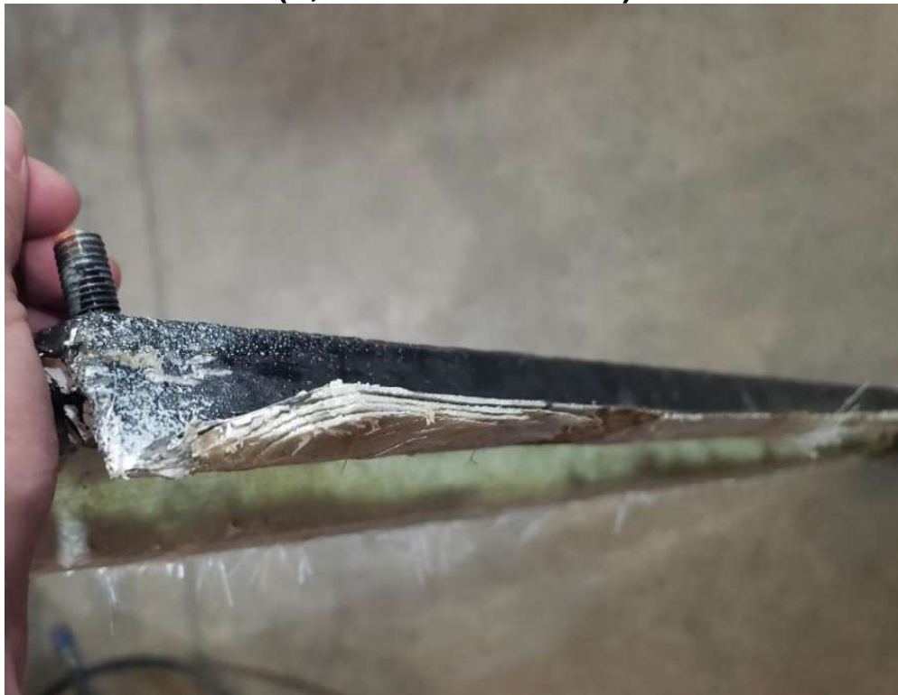
DAMAGED FRONT DOOR HAT BRACKET (6,494 TEST MILES)
