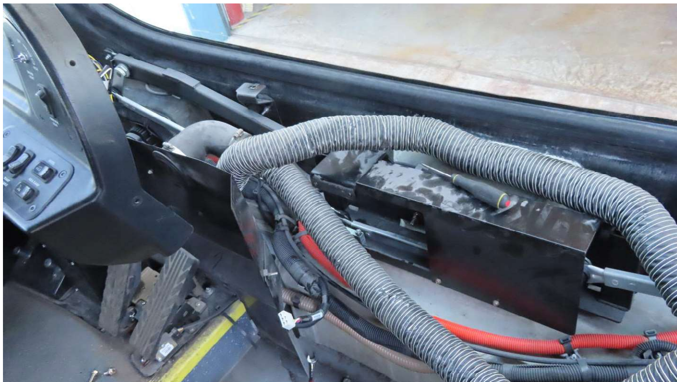
DASH PIECES REMOVED TO ACCESS WIPER MOTOR
