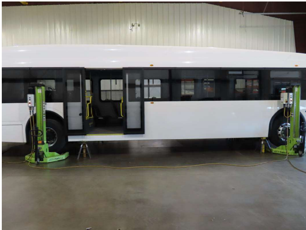
FRONT AND REAR JACK STANDS IN PLACE
