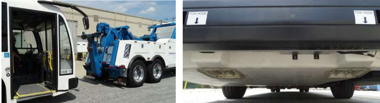
Figure 1-13. Tow Truck Positioned for Front Extraction
