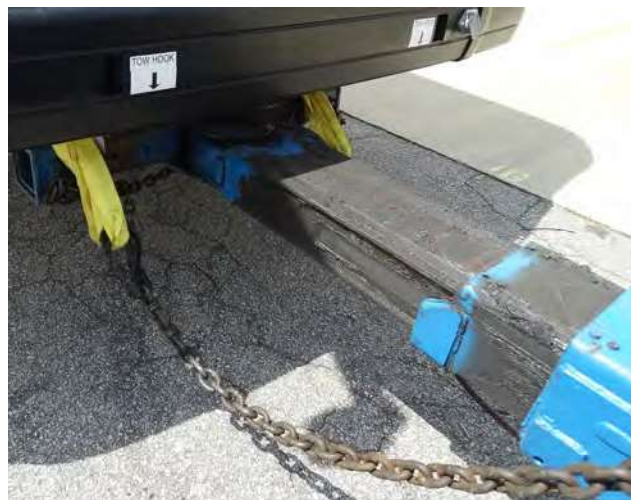
Figure 1-18. Install Tow Fork Safety Chains
