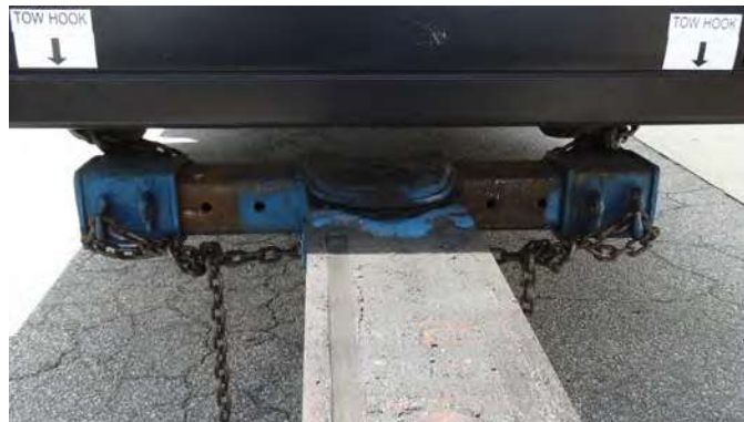
Figure 1-17. Install Tow Fork Safety Chains
